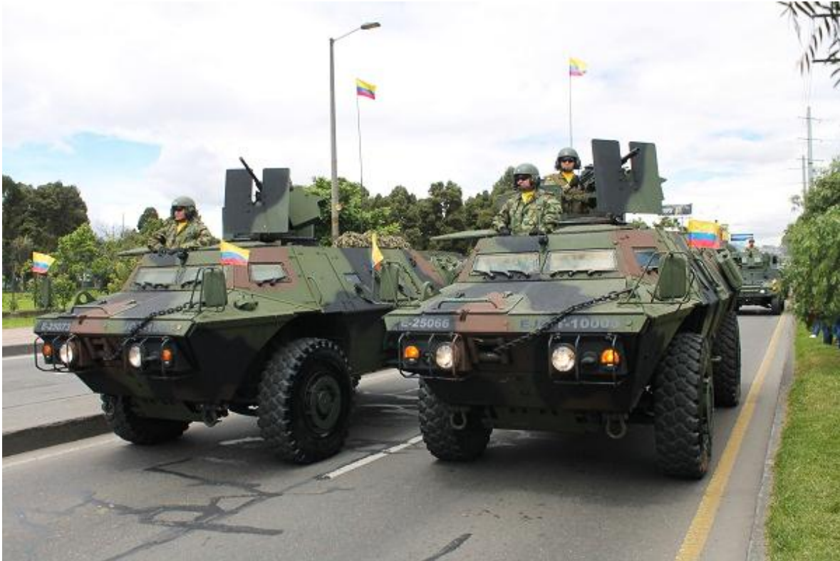
Armored M-1117 of American origin, in service with the Colombian cavalry. They are fitted with downgraded weapon stations, equipped with M2HB machine guns and Mk-19 grenade launchers.
