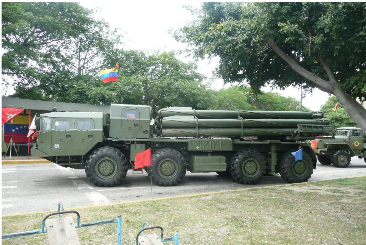
Smerch system launch vehicle in service with the Bolivarian Army of Venezuela. Photo from www.militaryforces.org
