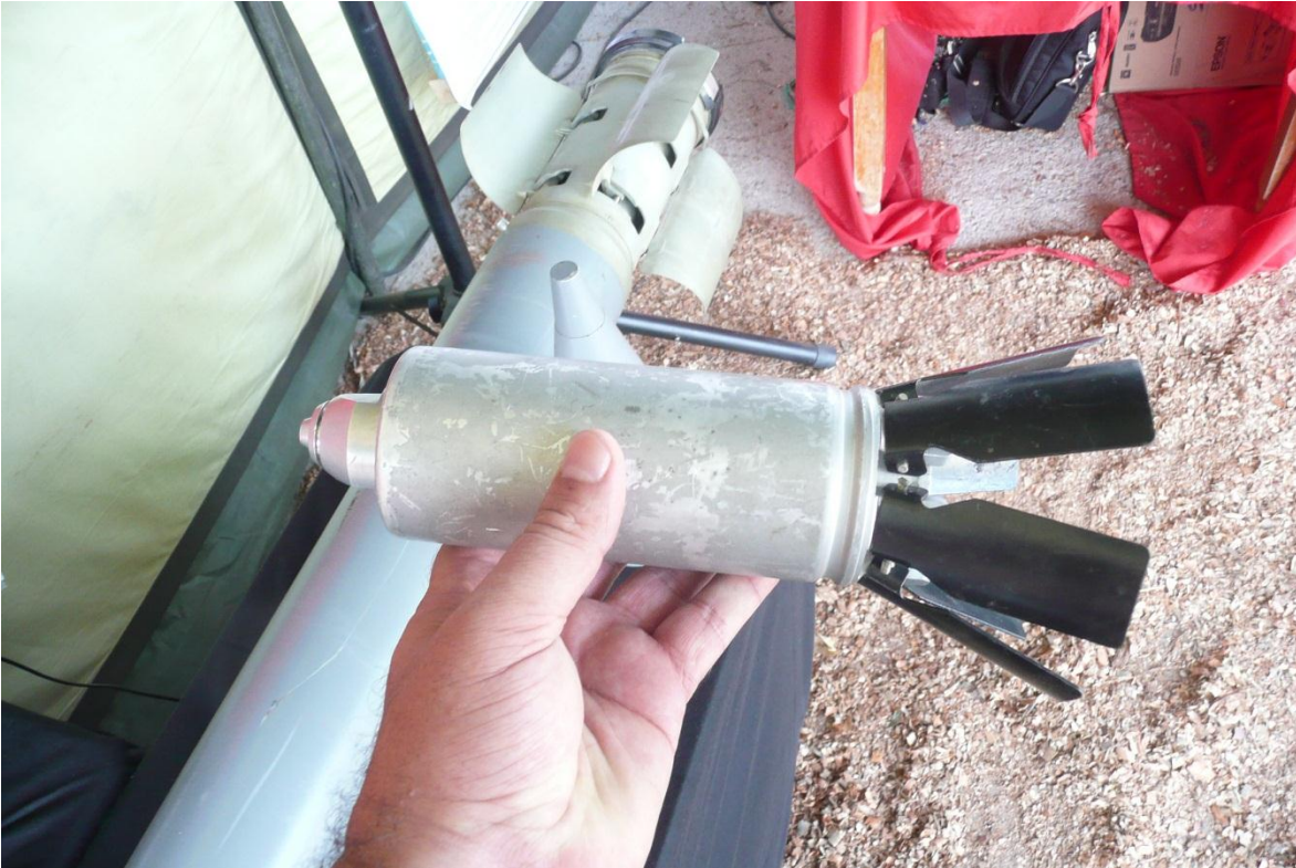
Submunition that is incorporated into the rockets of the Smerch system of Russian origin. Photo from www.militaryforces.org
